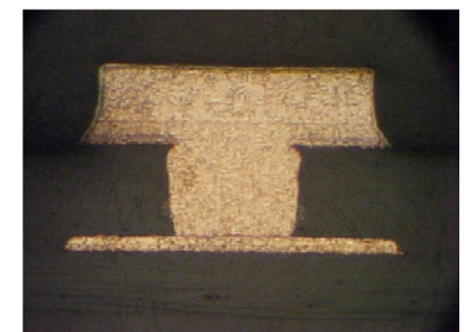
Etched and Solder Coated
